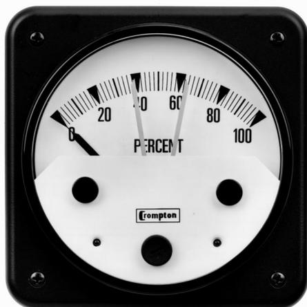
Series 077 meter relays combine a highly accurate indicator with High and Low set point relay. The relays can operate alarm and control devices when the monitored signal value moves outside the chosen set point limits shown by adjustable red index pointers.
